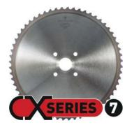
CX 7 is a Cermet tipped, PVD coated saw blade dedicated to cutting carbon steel (carbon content < 0.60%) with a low to medium tensile strength up to  $750 \text{ N/mm}^2$ . The best blade performance is being achieved when cutting lower tensile strength materials. On many applications, a blade life of  $50 \text{ m}^2$  and more can be achieved.
