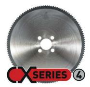
The high nickel content of austenitic stainless steel tubes makes them difficult to cut with HSS saw blades. With the dedicated tooth geometry of the carbide tipped and PVD coated CX 4 saw blade, perfect surface finish and burr-free tube ends will be achieved.
