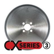
The CX 3 saw blade has been developed for cutting tubes on high performance automatic sawing machines, at a higher maximum cutting speed than with HSS saw blades. It is most effective on sawing machines with accurate control of chip load and variable feed rate. Bigger tips are applied at pitches > 9mm for added stability.
