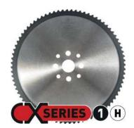
Applying a new saw body design, new tooth geometries and a new type of PVD coating, the CX 1-H saw blade has specifically been designed for cutting high tensile carbon steel  $> 900 \text{ N/mm}^2$ , carbon content  $\ge 0.60\%$ ) at very high production rates. It is also very suitable for cutting ferritic, martensitic and duplex stainless steel bars with a diameter larger than 35 mm.
