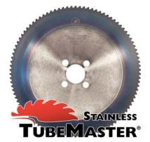
The TubeMaster Stainless saw blade has specifically been developed for cutting stainless steel tubes on orbital flying cut-off units. These saw blades can cope with cutting speeds between 60 - 120 m/min. TubeMaster Stainless offers high uptime due to a blade life up to  $3.5 \, \mathrm{m}^2$ , combined with high cut quality and production output.
