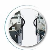
Compound cuts (pivoting and tilting) on both heads (45° x 45°)
